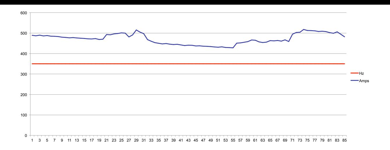
The graph above shows the current drawn by the pump on the initial test run, with operation at constant speed (35Hz output frequency). The time period of the test data is approximately 4 minutes, and shows the pump current drawn to be a minimum of 42.8 Amps, maximum 51.3 Amps, average 47 Amps.
