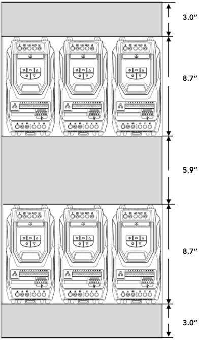
In both the above examples, the gray shaded areas above and below the drives are to be left free to allow air to easily enter and exit the drive cooling channel. No equipment may be mounted in these areas that would in any way restrict the flow of air into and out of the drive heatsink.
