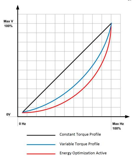
It can be seen that energy savings exist in the area between the different profiles. The Energy Optimization function adjusts voltage to provide energy savings under all conditions. Even a constant torque drive with energy optimization function can operate the motor more efficiently than a variable torque drive without energy optimization.
