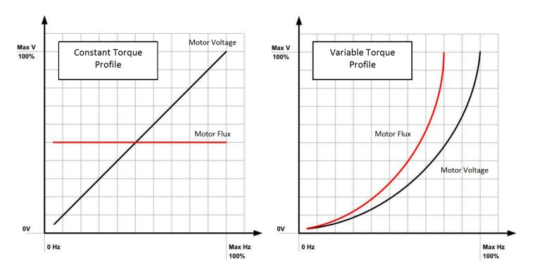
As its name implies, the constant torque voltage profile provides the best results in terms of energy saving when the load is constant and close to its nominal value. But under no load conditions the excess in magnetizing current would unnecessarily increase the losses in the stator making the motor less efficient.
